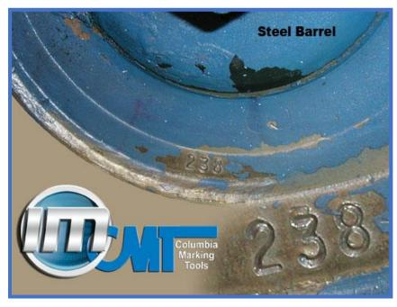
Nice sample mark of (3) 1/8" characters into a steel barrel.
