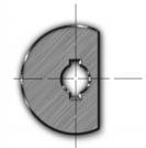
**5.** For marking parallel to axis of rounds and shafts. The concave surface of the roll die must have the same radius as the part.
